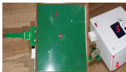
Figure 14. Components of a rapid U-value meter. Reproduced from Pekkala [103].
