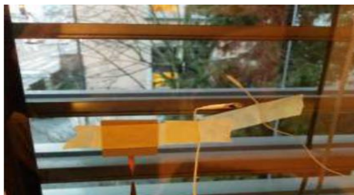
Figure 4. In situ measurement set-up for the glazing U-value determination using HFM method. Reproduced from [44].
