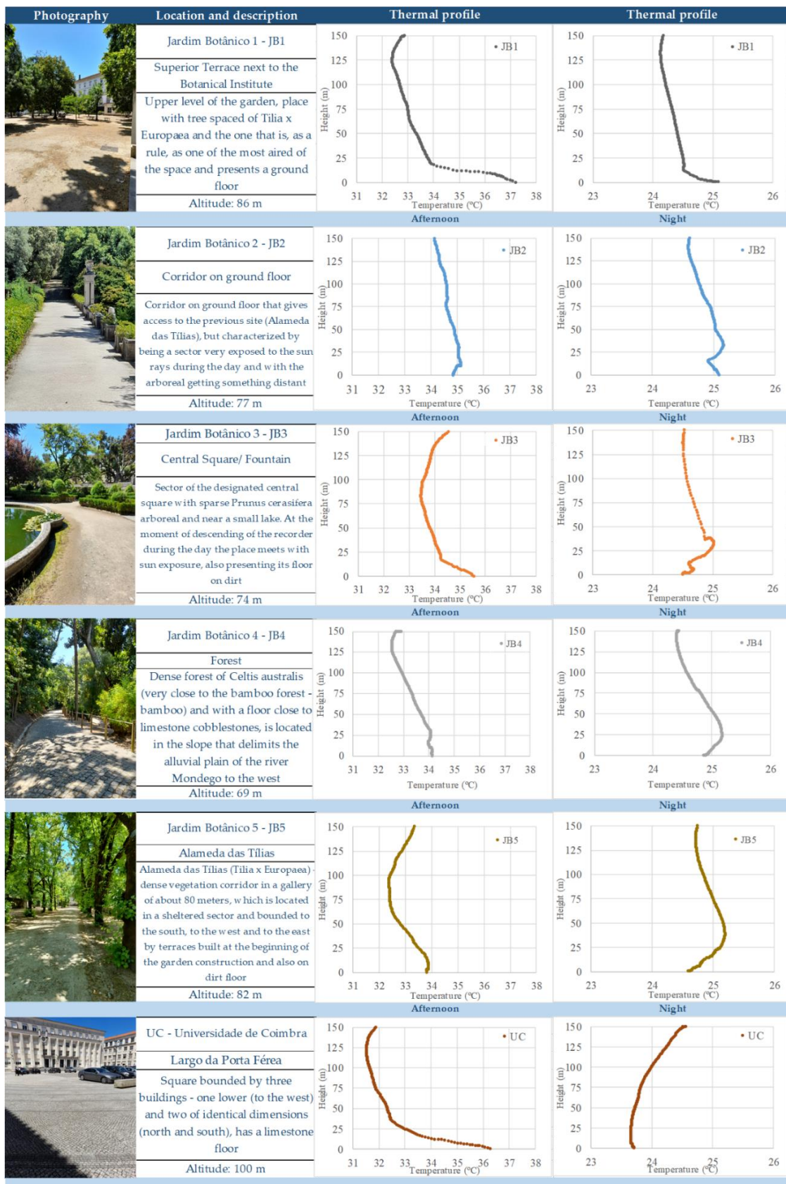
Figure 5. Characteristics of the surveyed areas under analysis, with the overlapping of thermal profiles taken from the Botanical Garden and the university building (27 May 2021).
