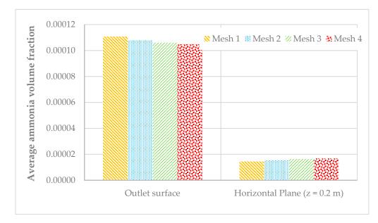
**Figure 3.** Average NH<sub>3</sub> volume fraction values at the global outlet surface and at z = 0.2 m plane, for the 4 tested meshes of the broiler building.
