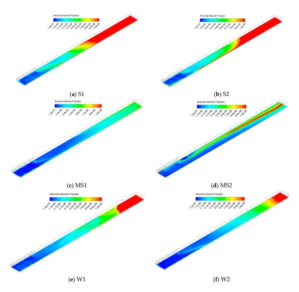
**Figure 7.** Color contours of  $NH_3$  concentration (volume fraction) in a plane at z = 0.5 m from ground, for the 6 configurations simulated in the broiler building.
