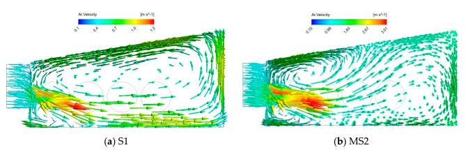
**Figure 6.** Vector profile in a plane yz, and at x = 15 m, for the configurations: (a) S1, and (b) MS2 in the broiler building.
