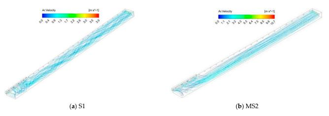
Figure 5. Streamlines for two configurations in the broiler building.
