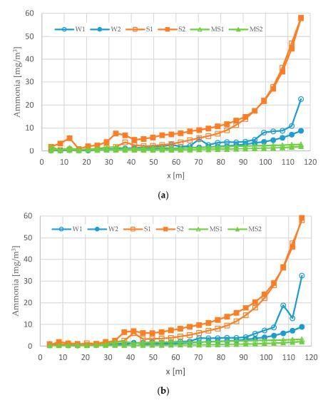
**Figure 9.** Ammonia concentration profile along the tunnel in a line (x direction), located at y = 7.5 m and at high of: (a) z = 0.5 m and (b) z = 1.8 m in the broiler building.
