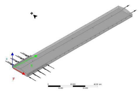
**Figure 1.** Geometry domain representative of the broiler building, with the inlet fresh air in the evaporative pad (lower left corner of the figure), and the outlet at the end of the tunnel.
