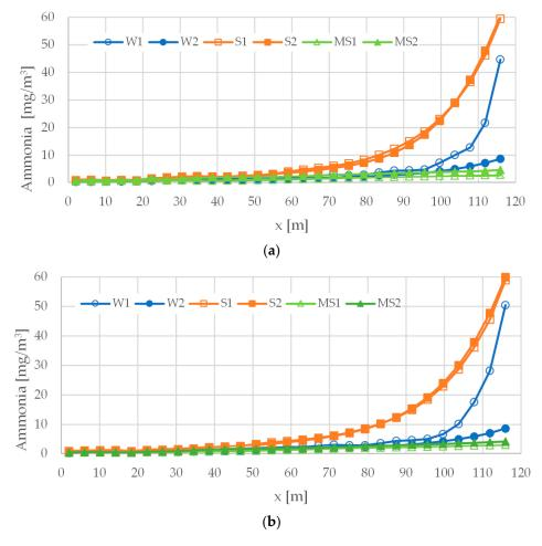
**Figure 8.** Average NH<sub>3</sub> concentration at each x location at height (**a**) z = 0.5 m and (**b**) z = 1.8 m in the broiler building.
