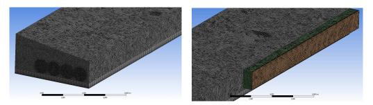
**Figure 2.** Details of the mesh, showing the mesh refinement at the outlet and inlet surfaces, in the litter and in the evaporative pad of the broiler building.
