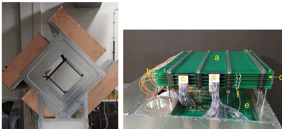
Fig. 1. Left panel: view of the arrangement of the detecting heads, forming a 30 cm wide cubic field-of-view. Right panel: detector stack, showing the readout electrodes (a), the connections for the timing/trigger amplifiers (b), the connections to the charge amplifiers (c), the RPCs (d) and a spare space for a future upgrade (e).
