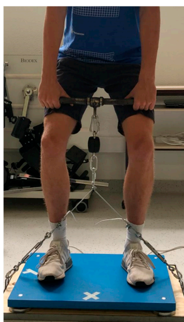
Figure 2. Placement of the Kistler platform on the system developed for this study.
