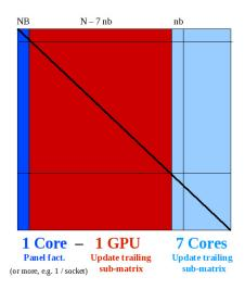
FIGURE 4. Load splitting for a hybrid LU factorization.
