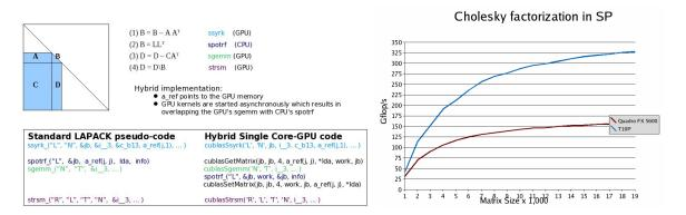
FIGURE 2. Left Looking Cholesky factorization: implementation (Left) and performance running the algorithm on an NVIDIA T10P and NVIDIA Quadro FX 5600 (Right) in single precision arithmetic.
