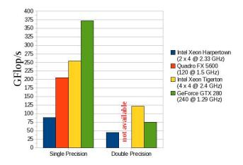
FIGURE 1. Peak measured performances of matrix-matrix multiplications on current multicore (from Intel) and GPU (from NVIDIA) architectures.
