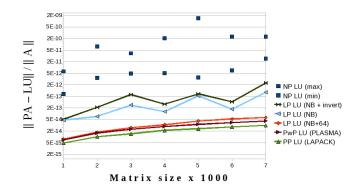
FIGURE 5. Accuracy of double precision LU factorizations on matrices of N(0,1) distribution.
