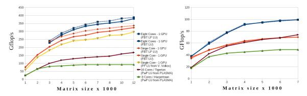
FIGURE 6. Performance for the RBT LU algorithm on a hybrid Intel Xeon  $(2 \times 4 \ @ 2.33 \ \text{GHz})$  – GeForce GTX 280  $(240 \ @ 1.30 \ \text{GHz})$  for correspondingly single (Left) and double (Right) precision arithmetic.
