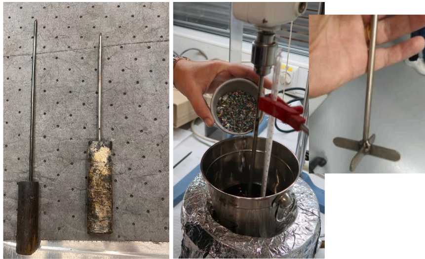
Fig. 4. Smooth rod (left) and mixing device for bitumen/recycled plastic (right).
