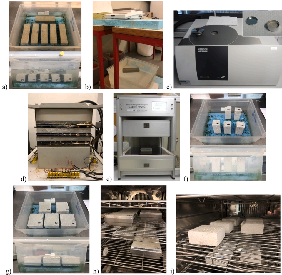
Fig. 2. Experimental campaign: determination of dry bulk density and saturation moisture content (a, b), specific heat capacity (c), thermal conductivity (d, e), water absorption due to capillary action (f, g), water vapour permeability (h), and sorption isotherm (i).
