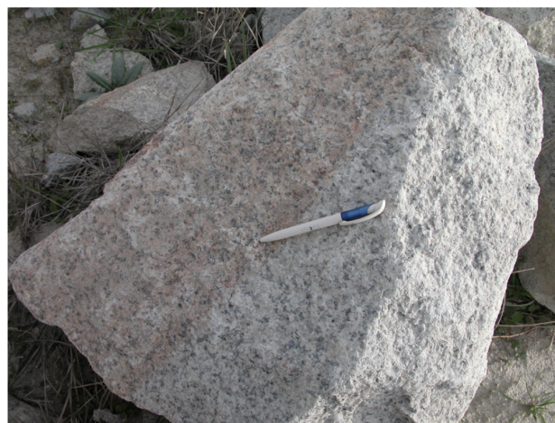
Fig. 5. Azul Platino and Amarillo Platino in the quarry. The latter is the weathered facies of the former.
