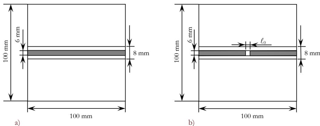
Figure 1: a) Control samples; b) Samples with different gap lengths ( $l_0 = 20$  mm).
