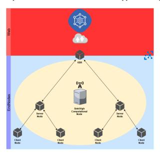
**Figure 1.** Architecture for intrusion detection in the context of Internet-integrated CoAP sensor networks.
