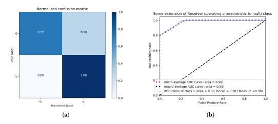
**Figure 9.** Binary class problem—Grid Search SVM with polynomial Kernel, One vs. Rest decision function shape, 30 iterations, with scoring criterion of accuracy, confusion Matrix (**a**) and ROC Curves (**b**).
