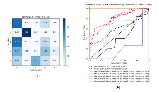
**Figure 6.** Multi-class problem—Grid Search SVM with: sigmoidal Kernel, One vs. Rest decision function shape, 30 iterations, and a scoring criterion of accuracy, confusion Matrix (**a**) and ROC Curves (**b**).
