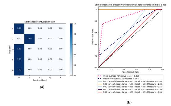
**Figure 8.** Multi-class problem—Grid Search SVM with sigmoidal Kernel, One vs. Rest decision function shape, 30 iterations, and a scoring criterion of accuracy, confusion Matrix (**a**) and ROC Curves (**b**).
