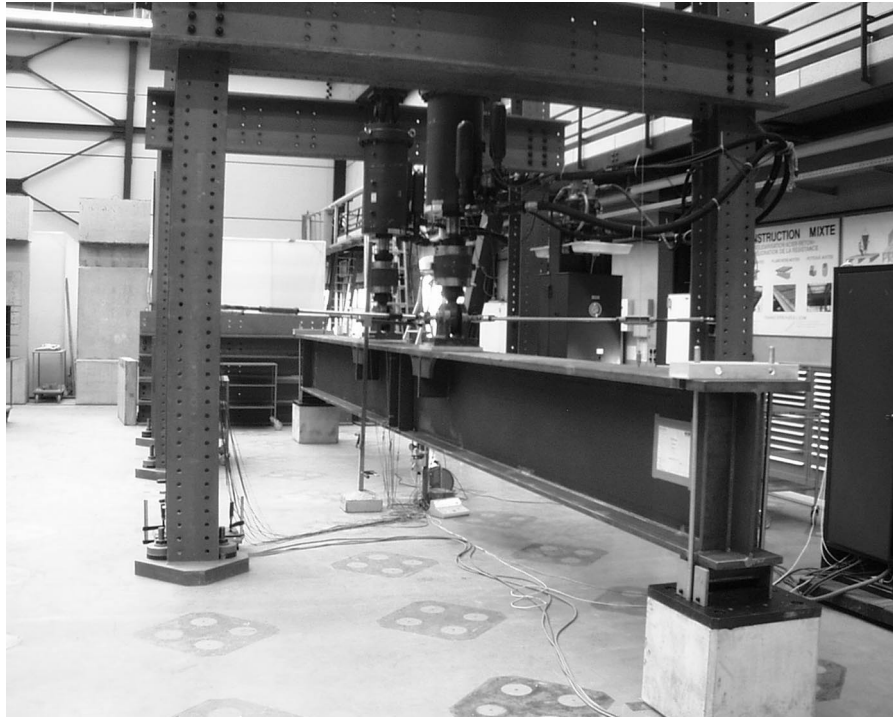
Fig. 5 Four-point bending tests on beams
