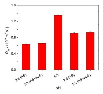
**Figure 1.** Tracer diffusion coefficients,  $D_T$ , of NH<sub>4</sub>VO<sub>3</sub> in saliva artificial (AS) at different pH values, at 25.00 °C. NaF represents sodium fluoride; pH = 6.5 is the value reached from the solutions obtained by dissolving NH<sub>4</sub>VO<sub>3</sub> in water.
