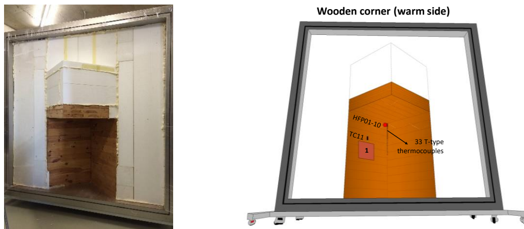
Figure 5. Photo of wooden corner (left), and diagram of the sensor layout (right), where 1 is an ultrathin flat plate heat flux sensor, HFP01-10 is a TRSY01 heat flux sensor, and TC11 is a TRSY01 thermocouple).
