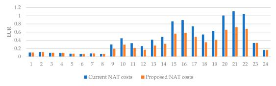
**Figure 7.** Comparison between the sum of hourly NAT costs for a 2-period Time-of-Use rate in a BaU scenario and in the proposed business model during the 6-month trial period. Source: Authors' own elaboration.
