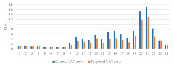
**Figure 8.** Comparison between the sum of hourly NAT costs for a 3-period Time-of-Use rate (3.45–20.7 kVA) in a BaU scenario and in the proposed business model during the 6-month trial period. Source: Authors' own elaboration.
