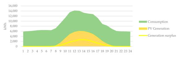
**Figure 10.** Sum of hourly photovoltaic generation, electricity consumption and surplus renewable generation from the 4 public buildings in Alfândega da Fé during the 6-month trial period. Source: Authors' own elaboration.
