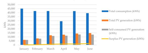
**Figure 3.** Distribution of total electricity consumption, total PV generation, parcel of self-consumed PV generation and resulting parcel of surplus electricity per month during the field trial period for Alfândega da Fé, Penela and Vila Real (Lordelo), respectively. Source: Authors' own elaboration.
