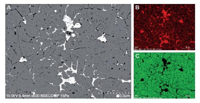
Fig. 10. A) SEM-BSE image showing the presence of Pb inclusions; B) EDS distribution map of Pb; C) EDS distribution map of Cu.
