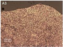
Fig. 11. Optical microscopy image showing the dendritic micro-structure of the three socketed arrowheads from Monte Figueiró (A1: arrowhead 1; A2: arrowhead 2; A3: arrowhead 3; cf. Fig. 3).
