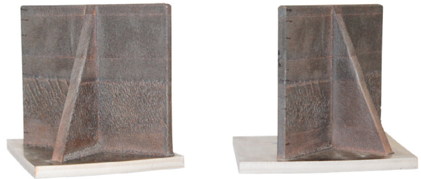
Fig. 11. Manufactured part using DED process.
