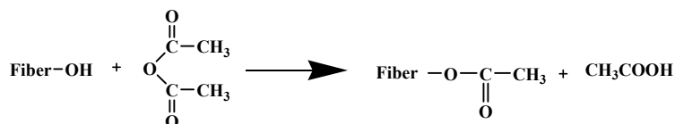
Figure 15. Chemical reaction of acetic anhydride with cellulose (Taken from reference [80] with permission of the Springer Nature).
