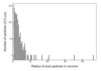
Fig. 3 Left: dust particulate size distribution from fluorescent image analysis of a witness plate. Particulates of size  $> 50 \,\mu$ m are rarely recorded. Right: dust particulate mass distribution of the same witness
