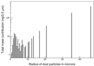
coupon showing contribution of particulate size to mass. Although most particulates are small, most of the mass on the coupon is from a small number of larger particulates
