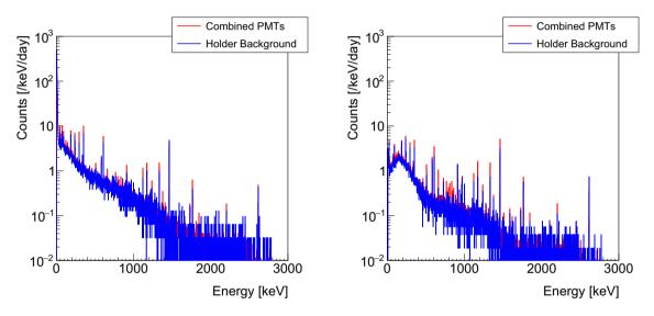
Fig. 5 Combined spectra for all R11410 PMT runs using Chaloner (left) and Lunehead (right) at the Boulby Underground Germanium Suite. In both cases, the background spectrum includes the holders used to secure PMTs in place in the detector castles
