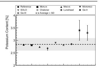
Fig. 1 Cross-calibration results for potassium concentration for the detectors used in the LZ HPGe radioassay campaign. The reference value for potassium concentration in this sample is  $(2.82 \pm 0.01)\%$ . Excluding this, an error-weighted mean of  $(2.84 \pm 0.02)\%$  was derived from the measurements of  $^{40}$ K. In this figure, the gray band represents the standard deviation of the measurements with a value of 0.25%
