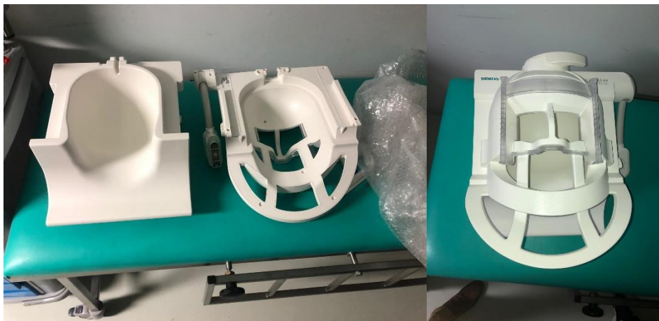
Figure 2.13 - Head/Neck 64 Coil, open (left) and closed (right), from Siemens.
