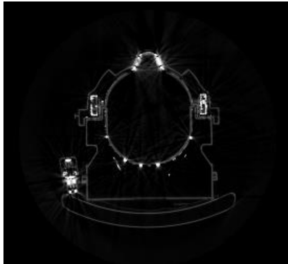
Figure 3.3 – Streaking artefacts in a plane of the CT scan of the Head and Neck 64 coil.
