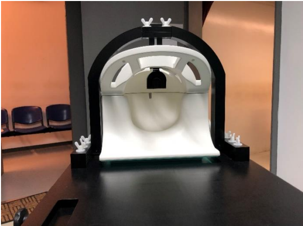
Figure 3.20 - Axial view for the preview of the final assembly between the immobilization device and the Head and Neck 64 coil.
