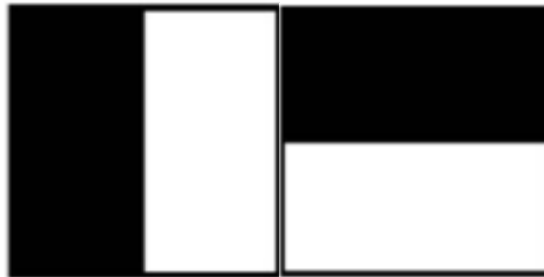
Figure 4.6 - Haar-wavelet horizontal (left) and vertical (right) types used for the SURF algorithm, From (Bay, et al., 2008).
