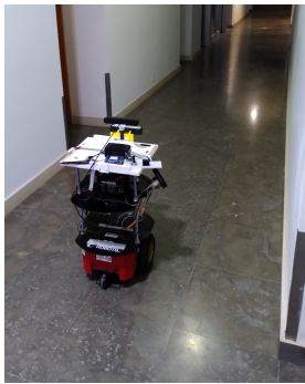
(a) System autonomously navigating through a corridor.
