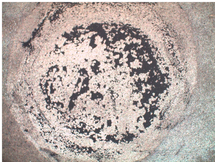
Figure 9. Top view of pulled-off area of an Ni-P plated PHNBR sample at 40 °C for 60 min.
