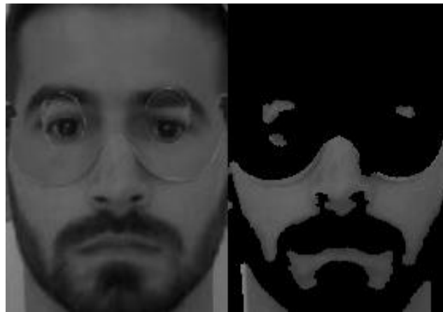
Figure 5. Original image ( left ) and the binary map ( right ), after applying the proposed skin detector.
