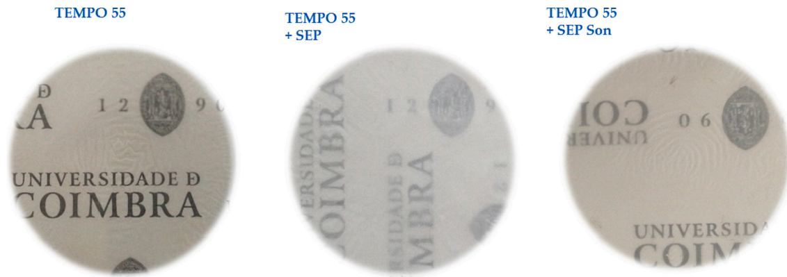
Fig. 4. Digital photos of TEMPO oxidised CNF-based films. Left – film obtained using neat CNF, without sepiolite; middle – composite film prepared with TEMPO-oxidised CNF and 20% sepiolite with the mineral dispersed using the high-shear disperser; right – composite film prepared with TEMPO-oxidised CNF and 20% sepiolite with the mineral dispersed using ultrasonication in the presence of CMC.
