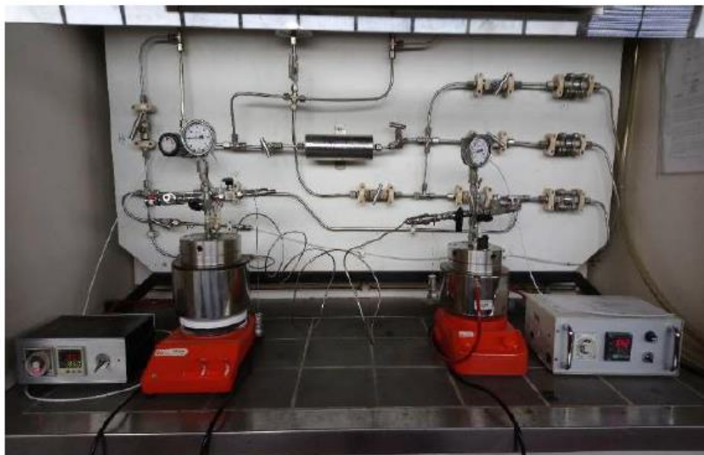
Figure 3.1. High-pressure system for catalytic reactions (Chemistry Department, University of Coimbra).
