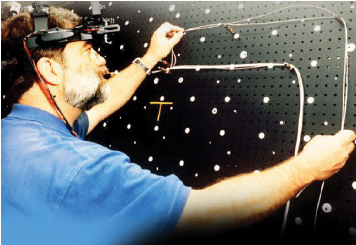
Figure 2.8: Researchers at Boeing using a see-through HMD to guide the assembly of wire bundles. Reference: [47]
