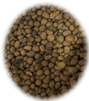
Figure 9. LECA of type S used in this study.
