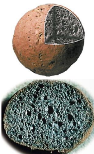
Figure 6. Image inside of a LECA particle, where pores of different sizes can be seen (Rashad 2018).
