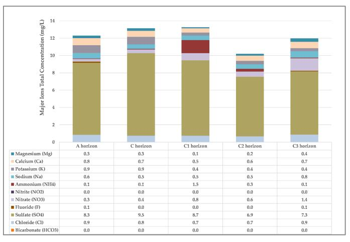
C3 horizons). On the other hand, sulphate was the main ion component in all samples, reflecting the mineralogy of the coal waste.
