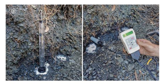
Figure 4. Field measurements of soil unsaturated hydraulic conductivity (a) and volumetric water content (b).
