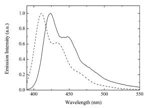
Figure 2. Normalized fluorescence spectra of PBS–PFP (6 mg  $L^{-1})$  in aqueous solution: alone (solid line) and with  $C_{12}E_5$  (5.3  $\times$   $10^{-4}$  M, dotted line).
