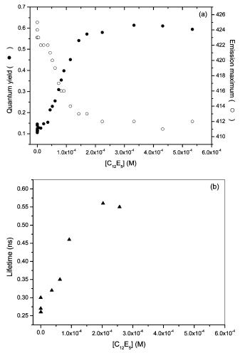
**Figure 3.** Changes in (a) quantum yield (bold circles) and emission maxima (open circles) and (b) fluorescence lifetime for aqueous solutions of PBS–PFP with  $C_{12}E_5$  concentration. For quantum yields, solutions were adjusted to have absorption  $\leq 0.1$  at excitation wavelength.
