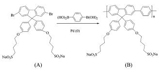
**Figure 1.** Synthetic scheme and structure of poly{1,4-phenylene-[9,9-bis(4-phenoxybutylsulfonate)]fluorene-2,7-diyl}.
