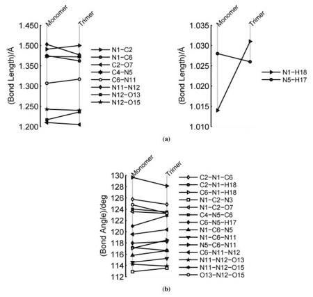
**Figure 7.** Comparison of (a) bond lengths and (b) bond angles for an isolated molecule and for a trimer of NIC3, computed at the level of theory B3LYP/6-31+G(d,p). Values for the trimer correspond to the central molecule.
