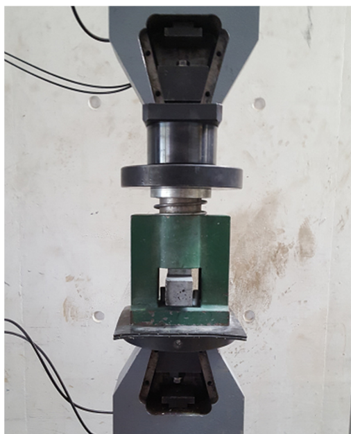
Figure 5. Compressive strength test set-up.
