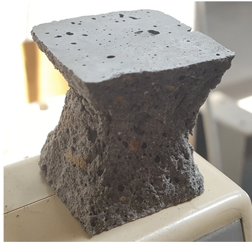
Figure 6. Fly ash-based AAB mortar specimen displaying conical semi-explosive failure.
