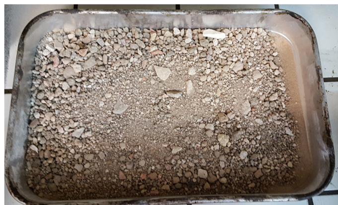
Figure 2. Dried construction and demolition recycled aggregates.
