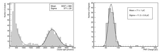
**Figure 5.** Distribution of the light content of the <sup>55</sup>Fe events reconstructed from the sCMOS images (**left**), and distribution of the charge measured by the PMT signals (**right**).
