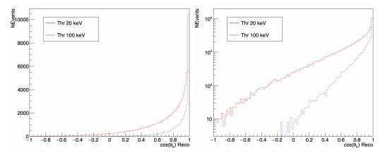
**Figure 16.** Angular distribution for electron recoils induced by solar neutrinos for 20 keV and 100 keV energy thresholds with a  $30^{\circ} \times 30^{\circ}$  angular resolution, shown on the right in log scale.
