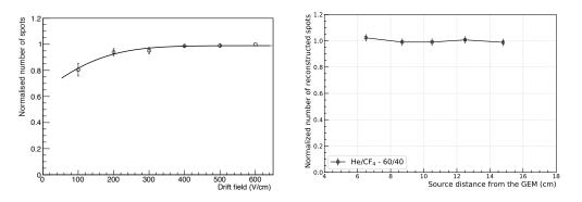
**Figure 6.** Behavior of the normalized number of <sup>55</sup>Fe spots as a function of the drift electric field (**left**) and event depth in the sensitive volume (**right**).
