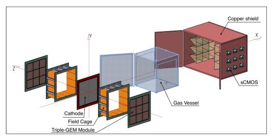
Figure 10. CYGNO PHASE\_1 Detector Layout.
