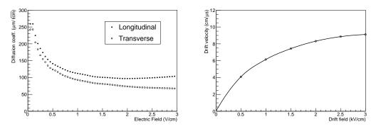
**Figure 1.** Transverse and longitudinal diffusion coefficients for  $\text{He/CF}_4$  60/40 (**left**) and electron drift velocity as a function of the drift field (**right**).
