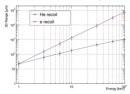
**Figure 3.** Average 3D distance between the production and absorption point for electron- and He-nucleus recoils as a function of their kinetic energy in a  $\text{He/CF}_4$  (60/40) gas mixture.
