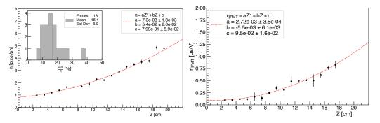
**Figure 7.** Dependence of  $\eta$  on the left and  $\eta_{PMT}$  on the right as a function of the track distance from the GEM (see text for details).
