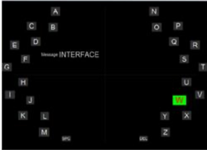
Figure 4.3: Lateral single character speller paradigm. Each symbol is highlighted once in each round. The highlight time of the stimuli is 75 ms with a 75 ms inter-stimuli interval and the inter-trial interval is 4s. [61]
