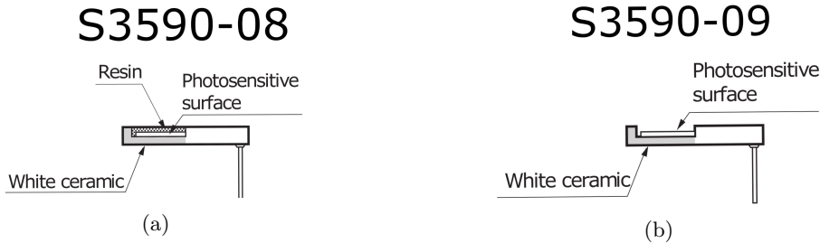
Figure 4.2: Scheme of the two photodiode models to be evaluated
