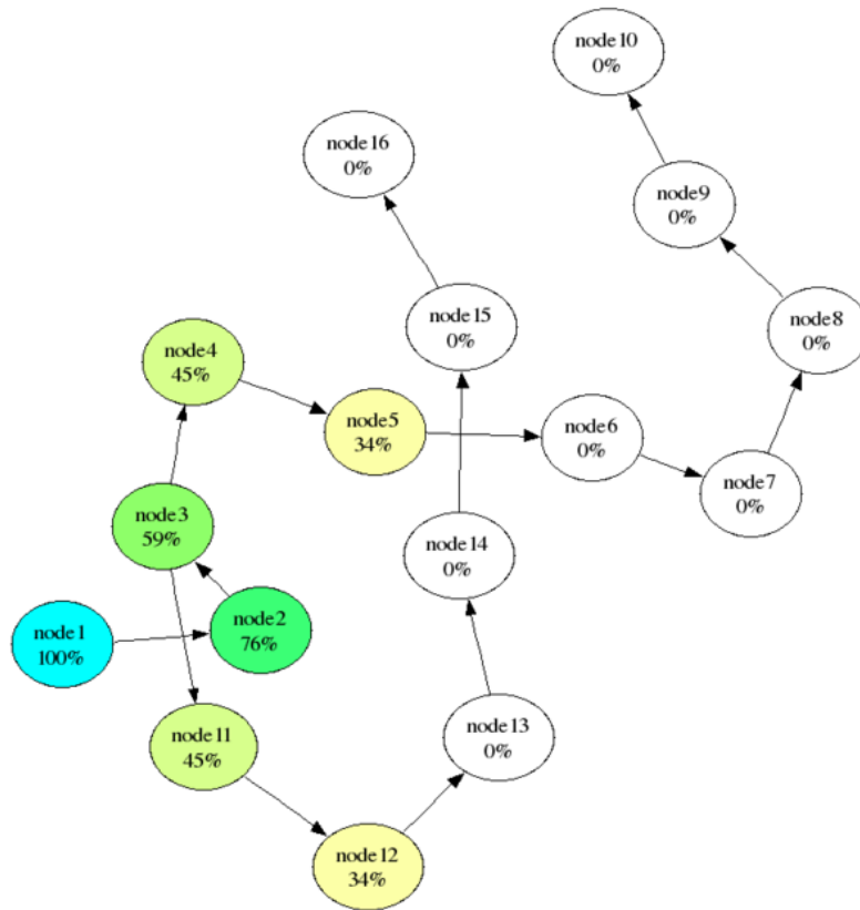
Figure 2.3: Example of spreading activation originated at node 1, with a weight of 0.9, for every link, and a decay factor of 0.85. Taken from Reed [2008]
