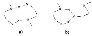
Figure 1. Ten- (a) and seven- (b) membered ring dimers of  $C_1E_1$  (schematic).
