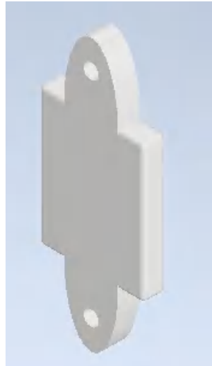
Figure 3.4: Sketch of the support where the layers were made - this support was also placed in the spin coater.
