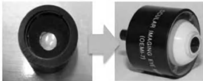
Figure 2.8: Result phantom, with the replicated retinal eye layers embedded into the commercial human eye model [31].
