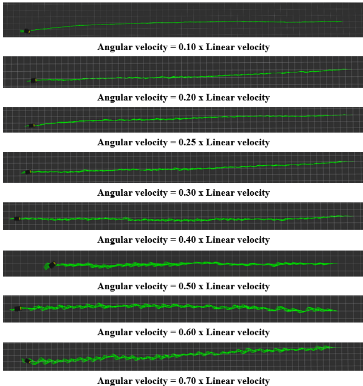
Figure 5.4 - Robot's trajectory considering the variation of the angular velocity.
