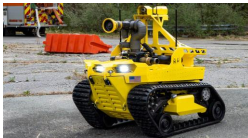
Figure 2.1 - Thermite RS1. Adapted from [2]
