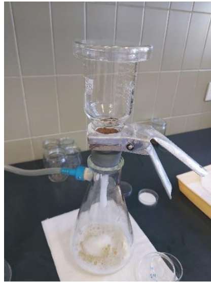
Figure 6 - Setup of the vacuum pump kit used to filter the samples. Column was always covered with a glass Petri dish to avoid any unwanted airborne contaminations of the sample filters. Control filter is opened near the working area shown (in the background).
