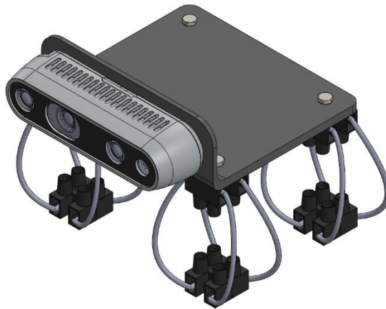
Figure 3.21 - Model of the WRI assembly to be used to reduce the D435i camera jello effect
