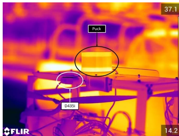
Figure 3.6 - Temperatures of the stereo depth camera (D435i) and the LiDAR (Puck) after the field test
