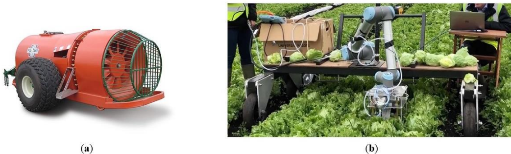
Figure 2.2 - Examples of robots used in agricultural applications: (a) PowerBlast 500 Gallon tree sprayer [24], (b) Vegebot [25]
