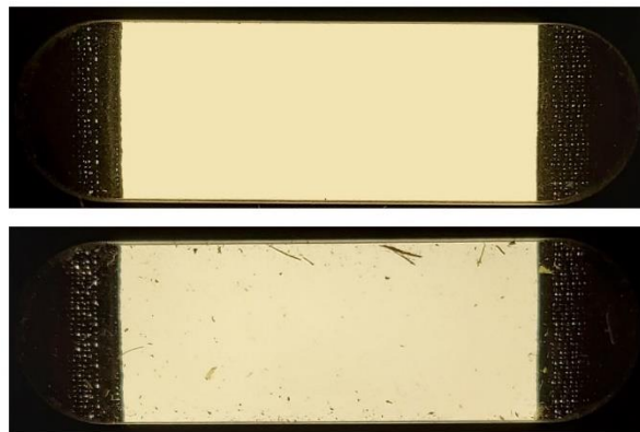
Figure 3.10 - Comparison of a clean glass panel (Top) and a glass panel with accumulated debris (Bottom)
