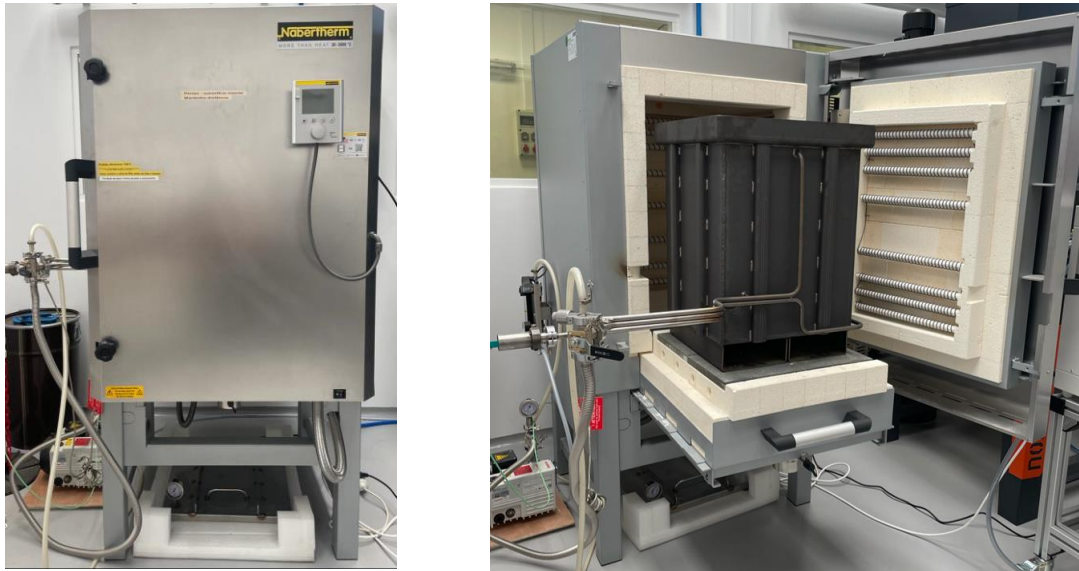
Figure 2.11. Oven Nabertherm NW200 used in the heat treatment of the cantilevers.
