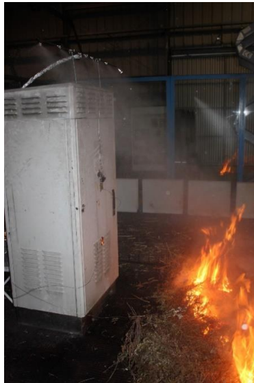
Figure 3.7 Water Mist Extinguish process.
