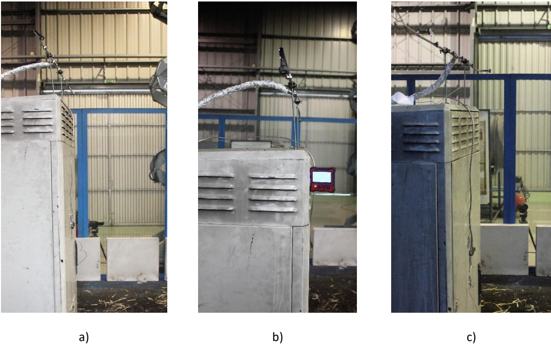
Figure 3.8 Sprinkler inclination at a) 45° (test 3), b) 0° (test 5) and c) 90° (test 6).
