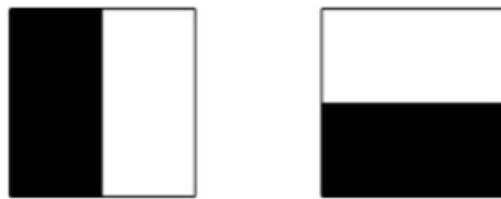
Fig. 3.9 Haar Wavelets for the x-direction and y-direction filtering responses. Black region weight is 1. White region weight is -1. Each wavelet response needs only six operations to be determined when used in conjunction with integral images.
