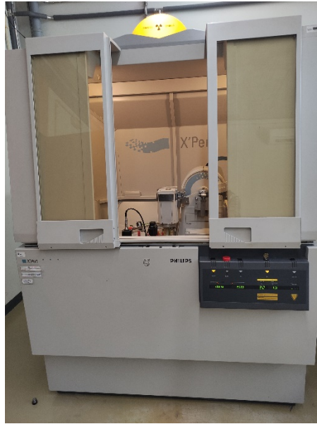
Figure 32: Philips XPert XRD equipment used in this work.
