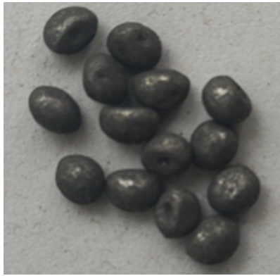
Figure 51: PLA granules coated with GNP and metallic alloy, as a typical example of the other coated systems.
