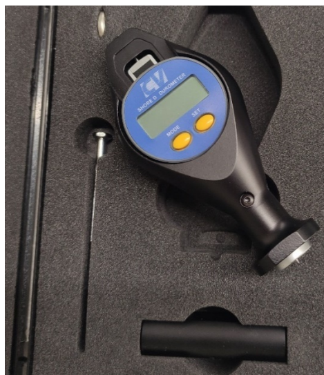
Figure 34: Shore (Durometer) Hardness Tester used in this work.
