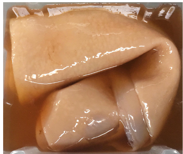
Figure 9 - Kombucha skin of 1m x 1m grown for 2 months using the biocouture recipe of Susan Lee for growing your own cellulose fabric garment prototype.
