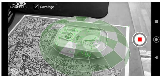
Figure 4.5: Using Vuforia Object Scanner to create an Object Data file.
