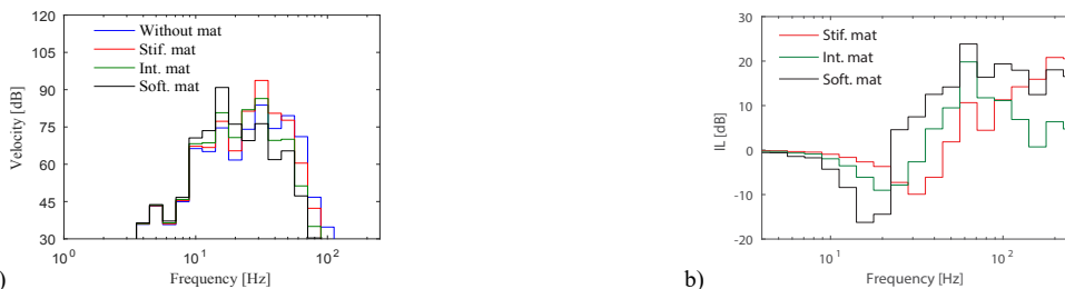
Fig. 4 – Frequency content of the vertical velocity at Point S1: a) one-third octave bands; b) Insertion loss curves (dB-ref 10^{-8} ).
