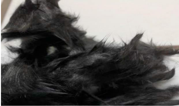
Fig. 1. Fiber dispersion aspect after ultrasonic bath and evaporation.
