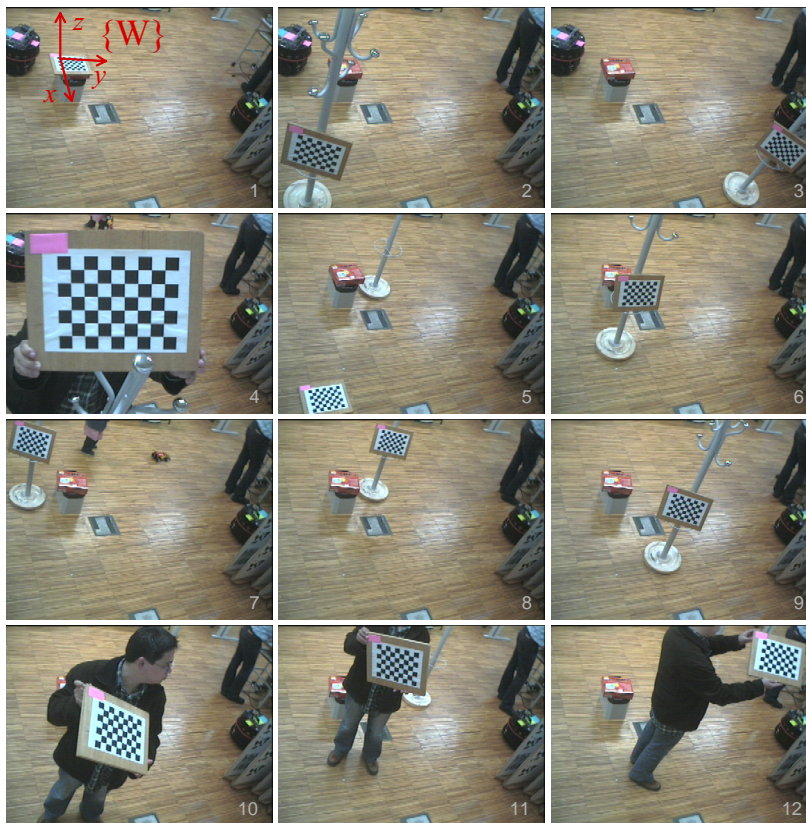
Figure D.2: Image set used in the calibration of the global camera.
