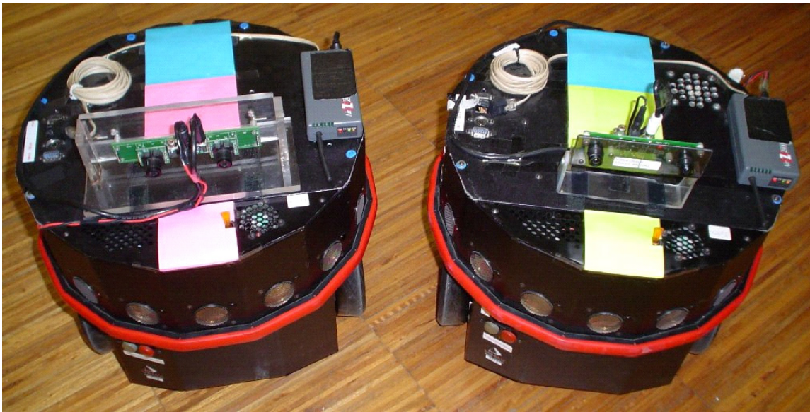
Figure 4.10: Scout mobile robots from Nomadic Technologies, Inc., equipped with sonars, stereo-vision and a modem radio providing TCP/IP wireless communication. Both robots have colored markers on the top (rectangular areas with different colors) in order to enable global localization, through color segmentation in the image provided by a global color camera covering the robots' workspace.
