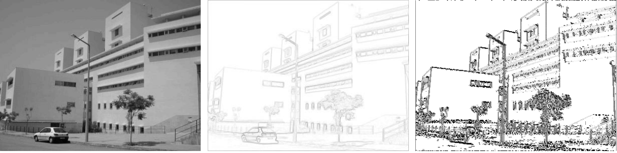
Figure 3.6: Original image, gradient magnitude and gradient phase at edges, obtained with modified Sobel edge detector
