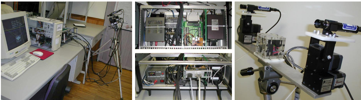
Figure 4.4: Complete system with host PC, hardware module, and stereo rig with inertial sensors mounted on a tripod
